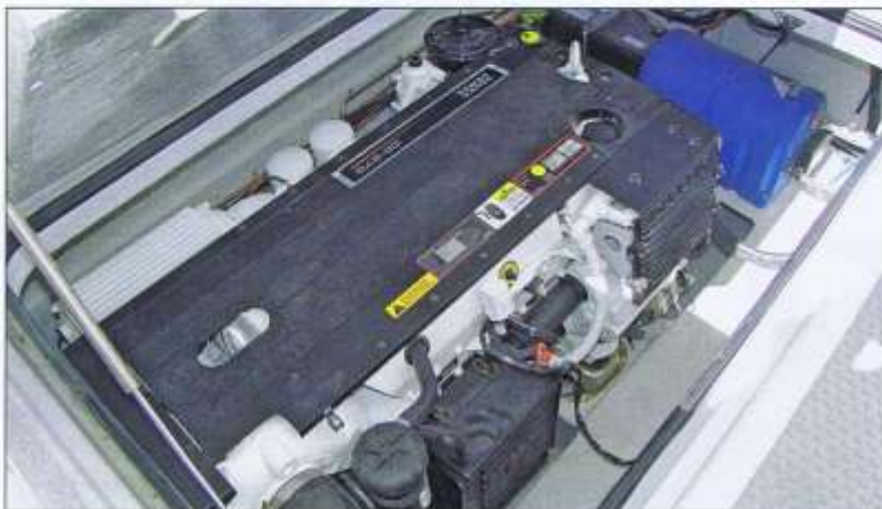
Performance of the new 370hp Volvo D-6 turbo diesels was superb, logging a very easy 34.6 knots and cruising at 20kn for just 52-53 l/ph.
