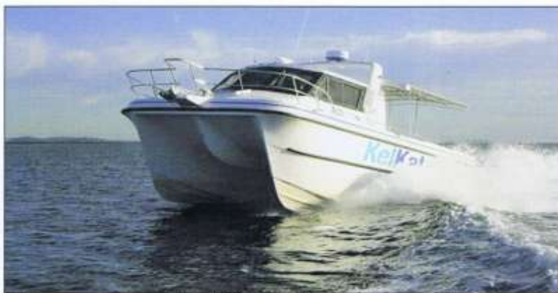
Performance of the new 370hp Volvo D-6 turbo diesels was superb, logging a very easy 34.6 knots and cruising at 20kn for just 52-53 l/ph.
